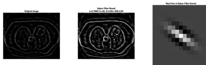
Figure 7. Applying Gabor Filter to Preprocessed Image
